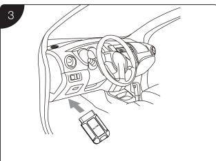
• Insert the MaxiVCI V150 into the vehicle's DLC, which is generally located under the vehicle dashboard.
